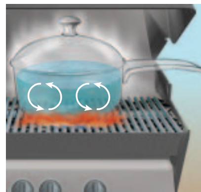
FIGURE D2.18 Convection transfers thermal energy through the movement of particles from one location to another.
