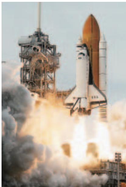
FIGURE A3.1 The space shuttle is driven by two chemical reactions. The main engines use liquid hydrogen and oxygen, and the booster rockets use solid fuel.
