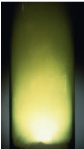
FIGURE A3.15 Burning sodium metal in chlorine gas produces solid sodium chloride.
