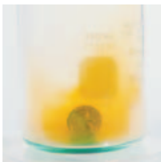
FIGURE A3.8 Evidence for the reaction between nitric acid and copper comes from the formation of bubbles, a yellow-brown gas, and a green or blue solution.
