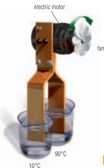
FIGURE B3.8 A thermo-electric converter is an example of a heat engine.
