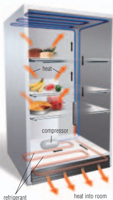
FIGURE B3.9 A refrigerator is a heat pump. Heat has to be pumped from inside the refrigerator to outside the refrigerator.
