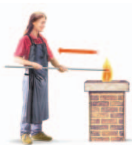
FIGURE B3.2 (a) Heat flows from the fire to the metal rod.
