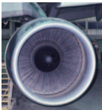
(a) The jet engine is an example of a heat engine.
