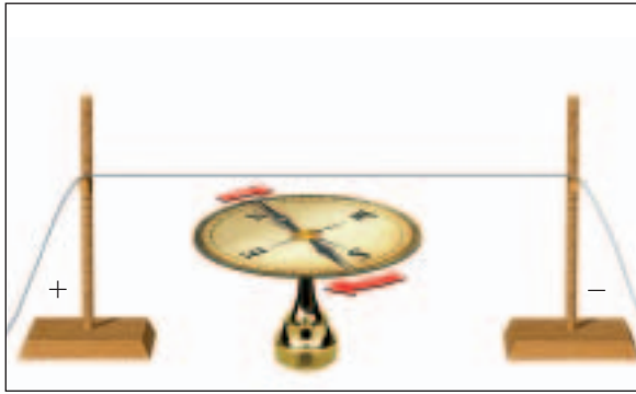
FIGURE B2.3 Oersted's experiment. As a metal wire with a current passing through it passes over the compass, the compass needle moves.
